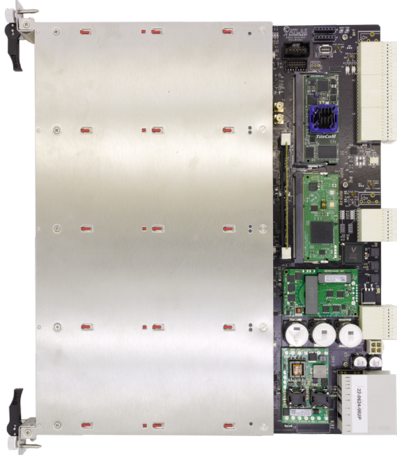
Figure 2.11: ACBB board version 1.2, including the TileCoM, IPMC and GbE switch mezzanine boards.
