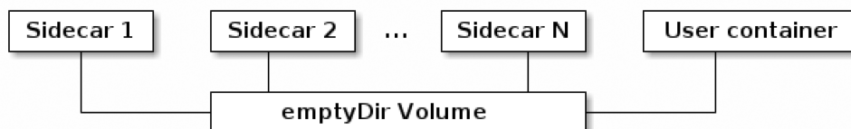
FIGURE 3 | The webhook creates and mounts an emptyDir volume shared by all the sidecars and the user container. This allows the sharing of data among all the containers in the pod.
