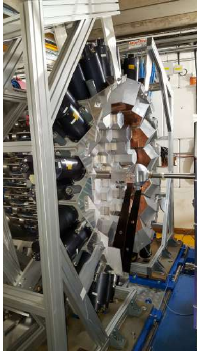
Figure 3.2: The NEutron Detector Array coupled to the Neutron Wall at 90^\circ [30].
