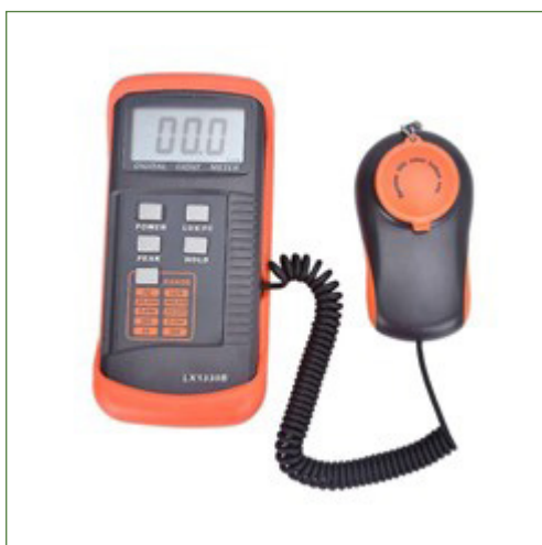
Figura 55: Luxómetro LX1330B Light Meter; Dr. Meter Digital Illuminance®.
