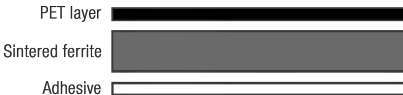
Figure 2.13. Layers structure of FSFS.
