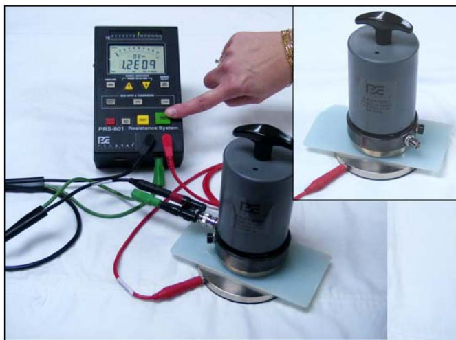
Figure 3.3. Measurement setup to determine the volume resistivity [12].
