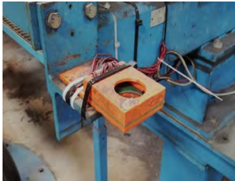
Figure 12. Actual PCB location for magnetic field measurement.
