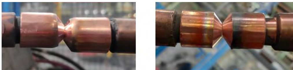
Figure 6. Types of electrode misalignment. Axial Misalignment-Angular Misalignment
