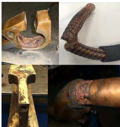
Figure 4. Real cases of wear in the secondary circuit
