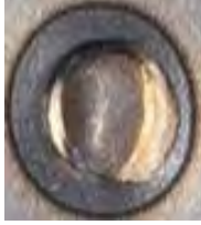
Figure 2. Poor-quality spot causes by misalignment.
