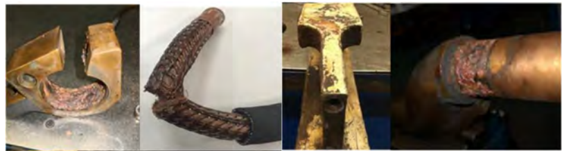
Figure 2. Typical wear in secondary circuit [15].
