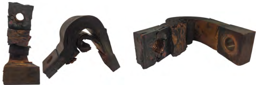
Figure 19. Real case of detection-worn copper strip. Cut sheets.
