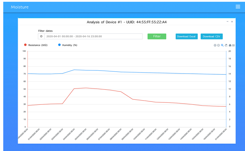
Figure 5.5: Web application device dashboard page showing the chart of moisture and resistance in function of time, the user can filter data by date and download it as Excel or CSV file.
