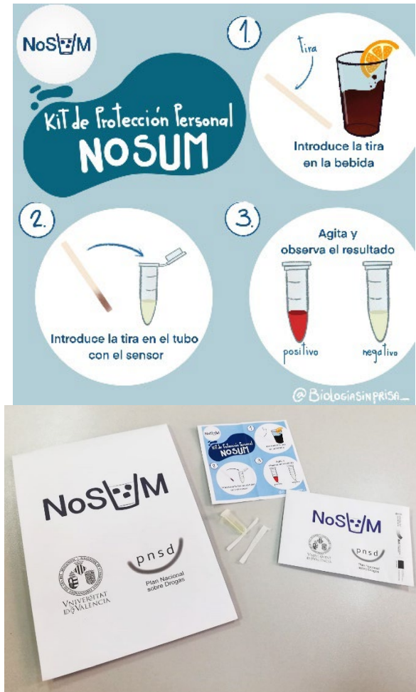
Figure A.5. Top) Instructions to use NoSUM. Bottom) Current appearance of the kit
