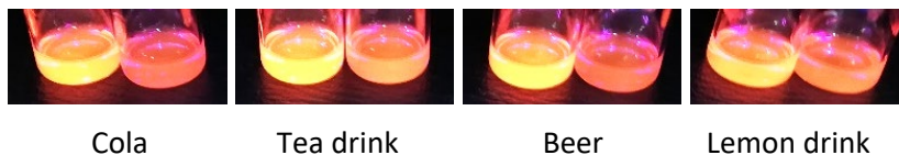
Figure S18. Changes in emission of probe 2 in the presence of NaGHB in soft drinks. Please notice that left vial means non-spiked drink, whilst the right vial stands for the spiked ones.
