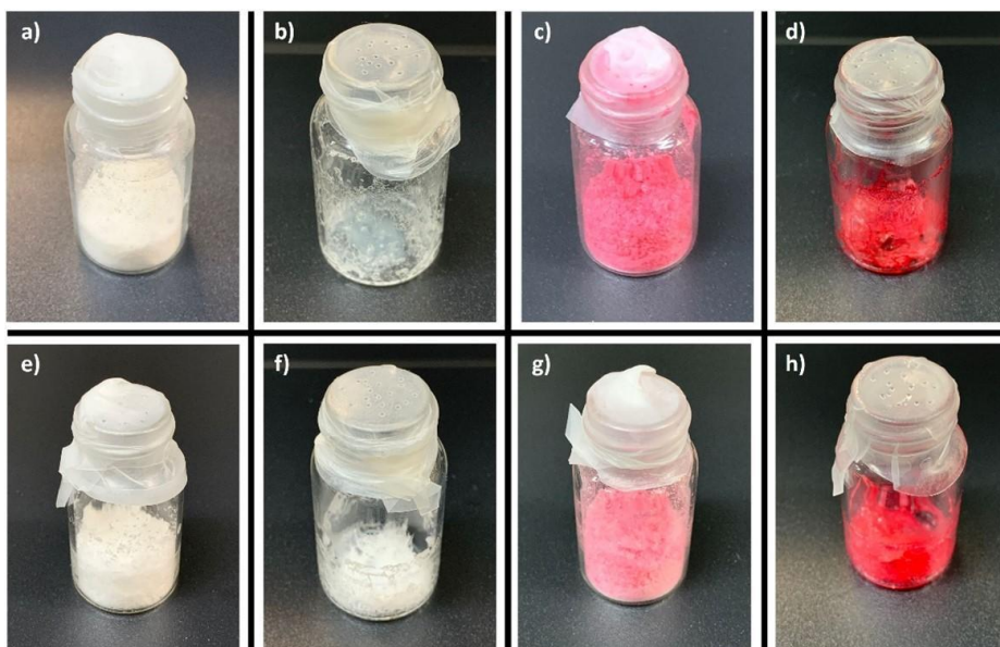
Figure 5.18. Representative photographs of freeze-dried B12-lipid vesicles: a) blank liposome-lactose; b) blank liposome-sorbitol; c) B12 liposome-lactose (L1); d) B12 liposome sorbitol (L1); e) blank transfersome-lactose; f) blank transfersome-sorbitol; g) B12 transfersome-lactose (T1d); h) B12 transfersome-sorbitol.
