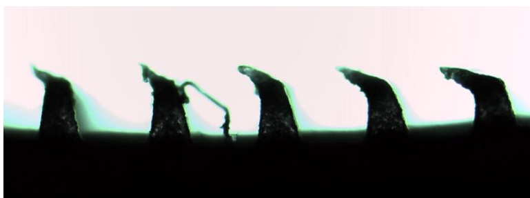
Figure 6.21. F9 deformed-needles after compression mechanical test.
