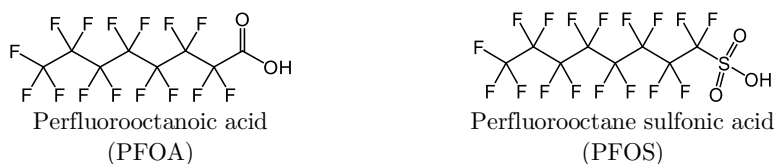
Figure 64. Molecular structure of PFOA and PFOS, as a representative example of the structure of studied PFCAs and PFASs respectively.
