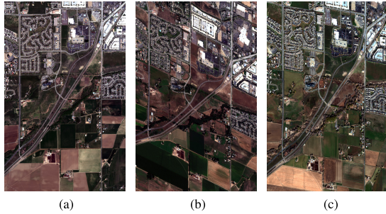
Fig. 6. Three WorldView-2 images present a wide variety of distortions due to both seasonality and view angle. In addition to the more obvious changes in agricultural and natural vegetation, the varying view angles result in variations in ground sample distances (GSD) of 2.0 m (May), 3.6 m (August), and 2.4 m (November). (a) May 2013, 14.0° off nadir. (b) August 2013, 43.6° off nadir. (c) November 2013, 29.3° off nadir.
