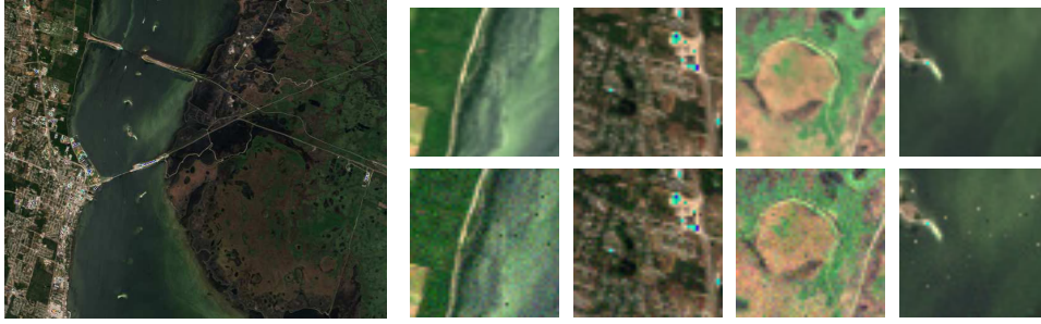
Fig. 4. (Left) AVIRIS hyperspectral image. (Right) Four illustrative chips of simulated changes. (Leftmost) Original image is used to simulate (Rightmost) an anomalous change image by adding Gaussian noise and randomly scrambling 1% of the pixels.
